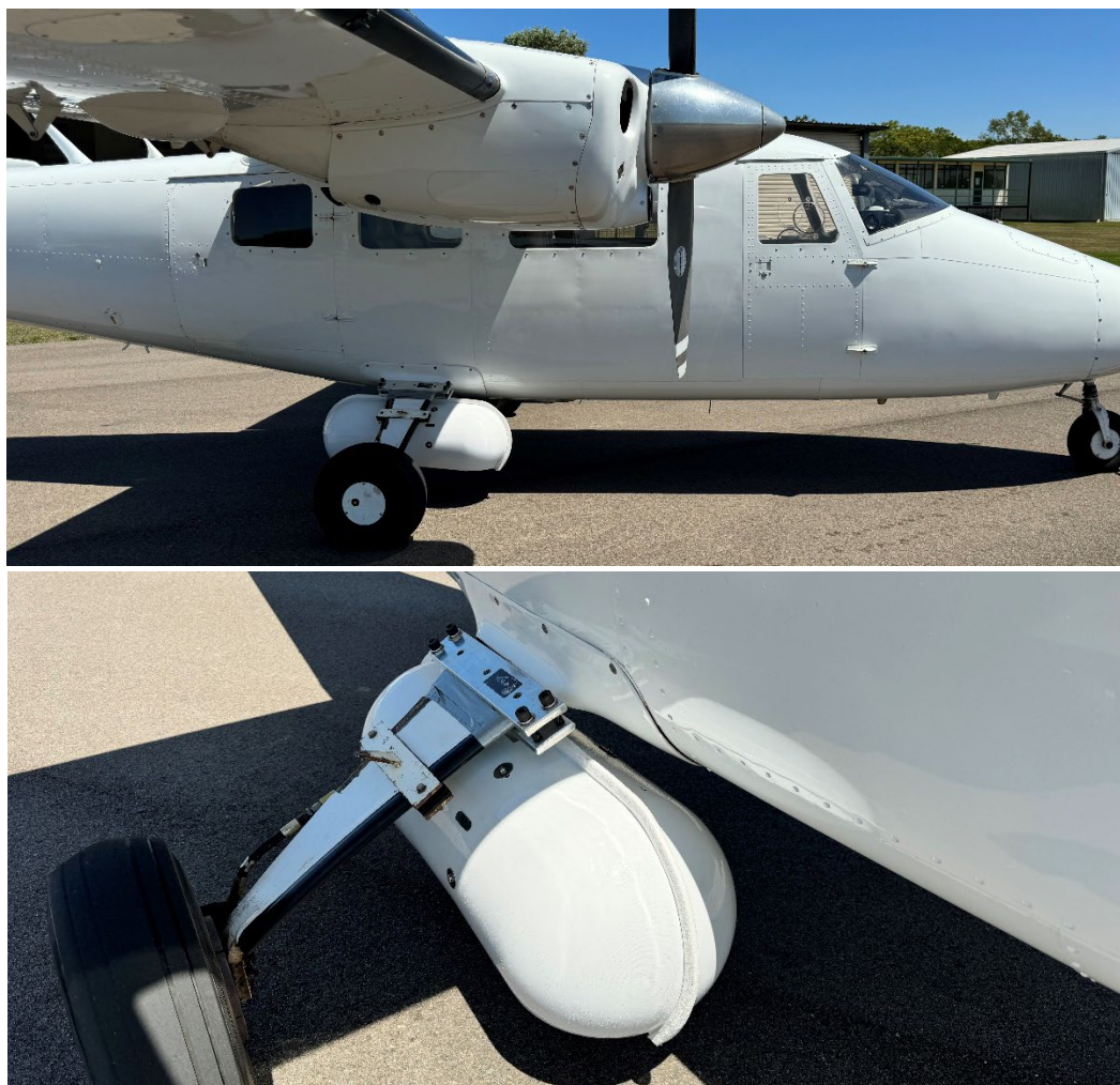
Figure 4 Manned aircraft with camera pods attached for aerial imagery © AeroGlobe Spatial Science
