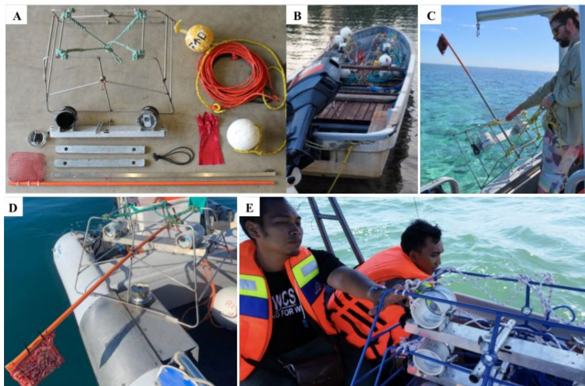
Supp Figure 2: Light weight stereo-BRUV. (A) Frame made of thin gauge stainless steel. Diode arm is passed through the back and front of the frame and not attached to the base bar. This reduces strain to the base bar during retrieval and allows the base bar to be made of light-weight hollow aluminum rectangular section (D). Base bar uses hooks and bungee cords to attach to the frame. The separation of cameras has been reduced to 500mm, with camera convergence of 5 degrees, to decrease the size of systems and making them easier for (B) travel with and use on smaller vessels and can be (C) hand-hauled. For research projects led by partners without
